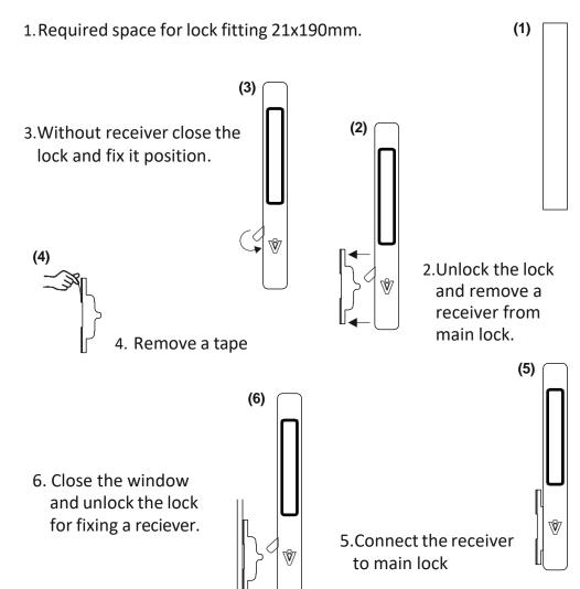
7. Drilling and fix receiver at his position.
